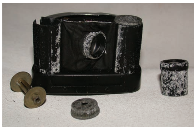
Figure 5. A pigeon camera, corroded objective and film reel before treatment. A thick white layer of corrosion is visible.
